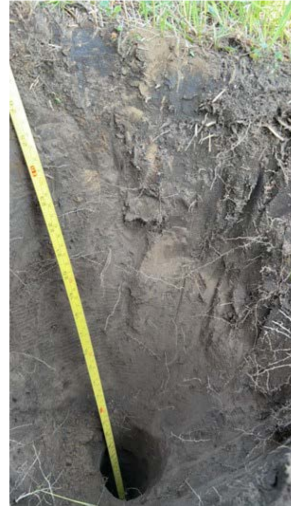
Photo of soil test pit
